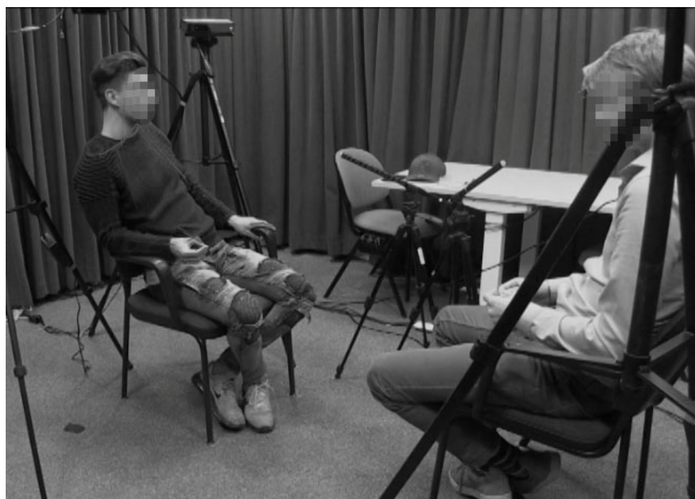
Figure 1. View of recording set-up as seen from participant A's (left) camera. Visible in this still frame is also one of the Microsoft Kinects, behind participant A's left shoulder, as well as the tripods for two of the other Kinects, and the two microphones (center).
